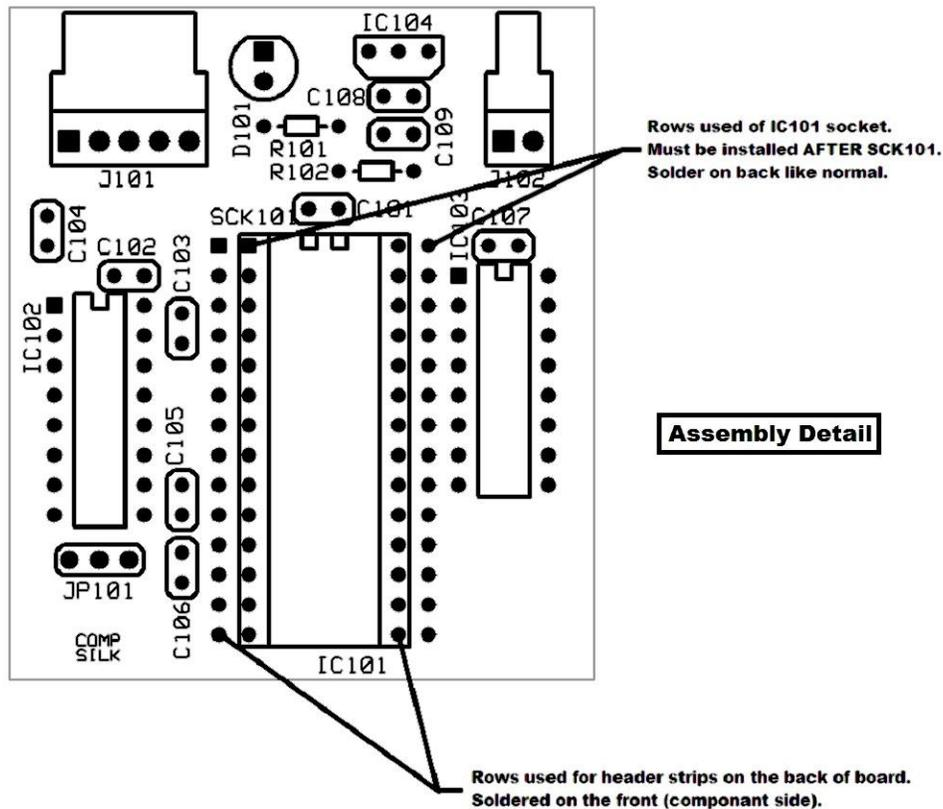
NOTE: Two 14-pin sip header strips need to be installed on the solder side (bottom) at location SCK101. It is through these 28-pins that the daughter board will plugged into the H8-5 board at location IC123.
